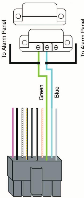
**Figure 5** Shunting a Normally Closed Zone
