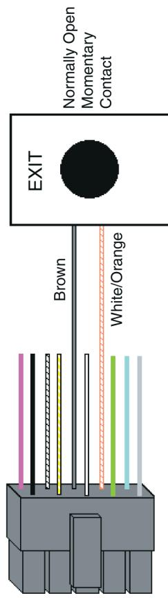
Figure 6 Wiring a REX Button
