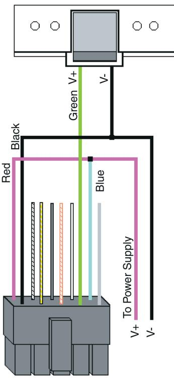
**Figure 4** Wiring 212e Keypad to Electric Strike
