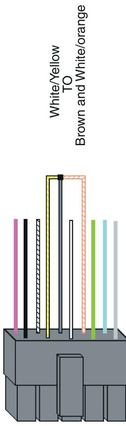
**Figure 7 Programming Mode Loopback Standalone**
