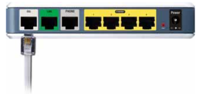
Figure 4-1: Connect the ADSL Line
