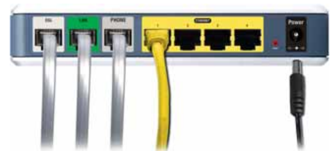
Figure 4-5: Connect the Power
