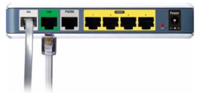
Figure 4-2: Connect the Voice Line
