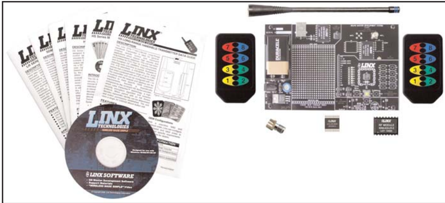
Figure 8: OTX-***-HH-CP8-HS Master Development System
