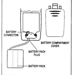
Remove the HANDSET BATTERY COMPARTMENT COVER by sliding it down.
