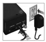
Plug the power supply's cable into the Base-1L's power input, then plug the power supply into a properly grounded wall outlet (110 volts, 50/60 cycles).
