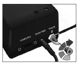
Connect a wire between the Command Base's binding post and the common (U) terminal on all transformers powering your track. You can also connect the wire between the Base-1L and the outside rail of your track. (Connect the wire to both outside rails if you use hi-rail track.)
