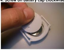
5. Screw cap on clockwise until it stops and cap is level with transmitter case bottom
