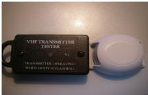
8. Tester light will activate when placed on top of running transmitter
