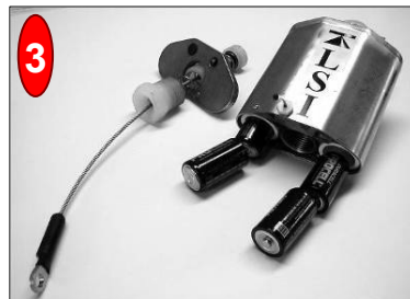
Figures: Changing batteries of a GS050 anti-two-block switch
