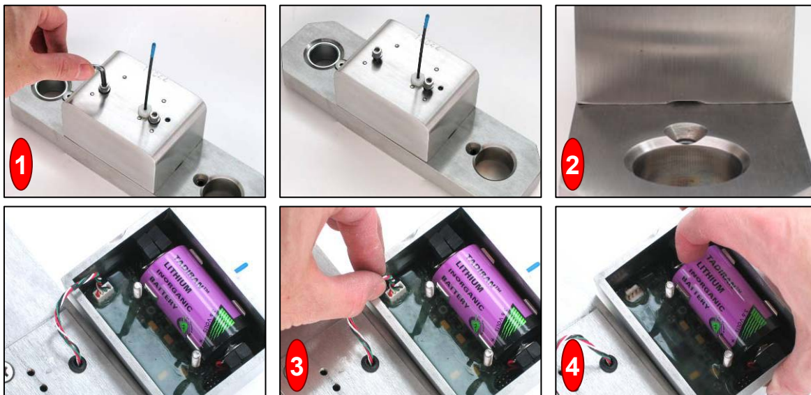
Figures: Removing the old battery
