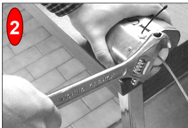
Figures: Changing batteries of a GS050 anti-two-block switch
