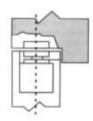
A cut for the arm is required on the stop side of the door only. A hole must be drilled for the control know of the No. 1 Series holder only.
