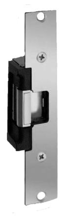
The 7000 series has a modular design to accommodate both cylindrical and rim exit locksets. The 7000 series will accommodate various types of latchbolts from 5/8" to 3/4" throw. The unique design of the keeper module allows the unit to operate under excessive door loading. The 7000 series has an internally mounted solenoid for ease of installation in metal, aluminum and wood jambs. The heavy-duty construction of the 7000 series electric strikes makes them ideal for high usage applications.
