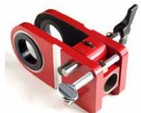
**Gator Grip Pads** These pads are a self adhesive back neoprene with a textured gripping surface that virtually locks the jig to the door, minimizing the possibility of slipping when properly clampted to the door. **Standard on the BUL-2.**
