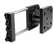
This rugged tool is hardened throughout and covers the widest range of locksets possible. It works equally well on metal or wood doors when using the proper drill bits and will also locate the anchor plate lug holes. Can handle doors 1 1/8"-2" thick and will work any backset from 2 3/4"-5".
