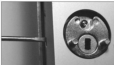
Fig. 7a: Tighten the interface cylinder set screw
