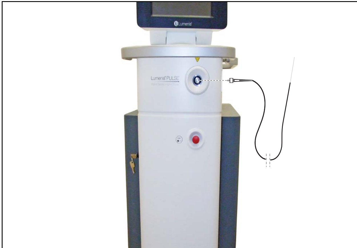
Figure 7: Connecting the Optical Fiber
