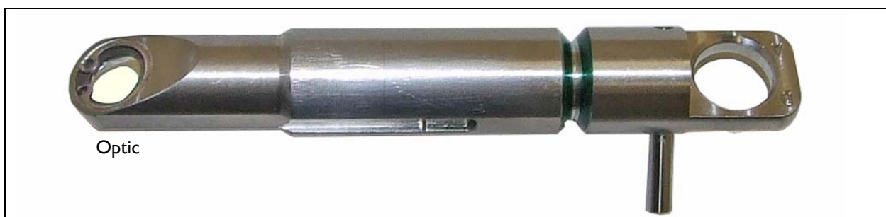
Figure 15: Inspect the Debris Shield Optic
