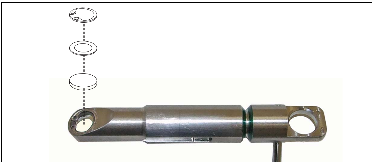
Figure 17: Change the Debris Shield Optic
