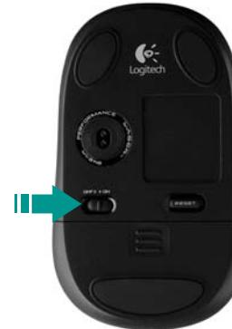
**English** Turn on mouse. Slide the switch on the bottom of the mouse. When you are traveling with your mouse or will not be using it for a long period of time, turn the mouse off to extend battery life.
