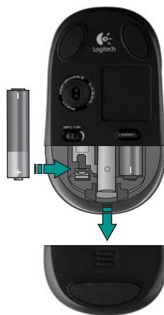
**English** Install the AA alkaline batteries. The LED will blink red when the batteries need to be replaced.
