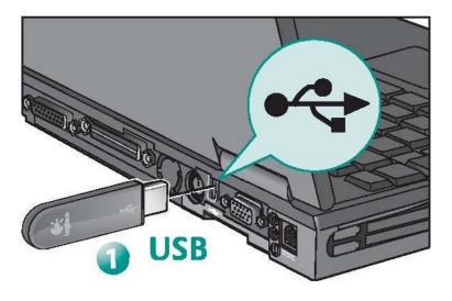
**English** (1) Plug wireless mini-receiver directly into computer's USB port. **Optional.** Use USB stand for convenient access to wireless mini-receiver or for better wireless reception. (2) Plug USB stand into computer's USB port. (3) Insert wireless mini-receiver into USB stand. **Optional.** A PS/2 adapter is provided for PS/2 connections.
