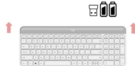
Show that if that forehead is slid upwards a dongle and battery compartment will be found inside
