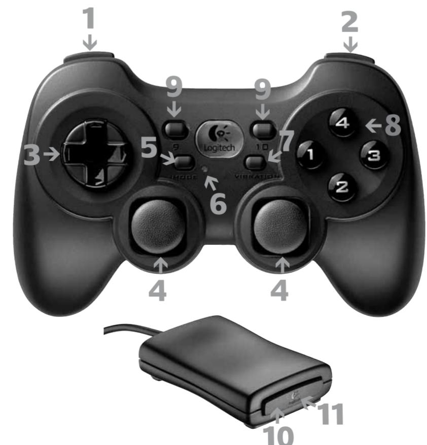
**ENGLISH** 1. Two left triggers 2. Two right triggers 3. D-pad 4. Two analog sticks with programmable buttons (press down to activate) 5. Mode button (selects flight or sports mode) 6. Mode/status light 7. Vibration button (turns on/off vibration function) 8. Four primary programmable action buttons 9. Two secondary programmable action buttons 10. Receiver Connect button 11. Receiver Status light
