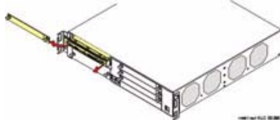
Figure 7. Clear the left side of the G700 Media Gateway
