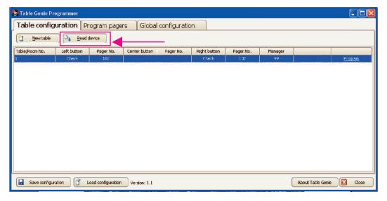
While holding the programming cable in place, click 'Read Device'.
