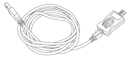
Connect the complete programming cable to an available USB port on your computer.
