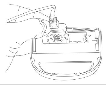
4. While holding the programming cable in place, click on the 'Program' link for the desired table.
