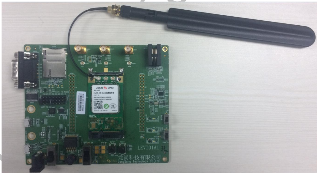
Figure 6: Antenna transit cable connection view
