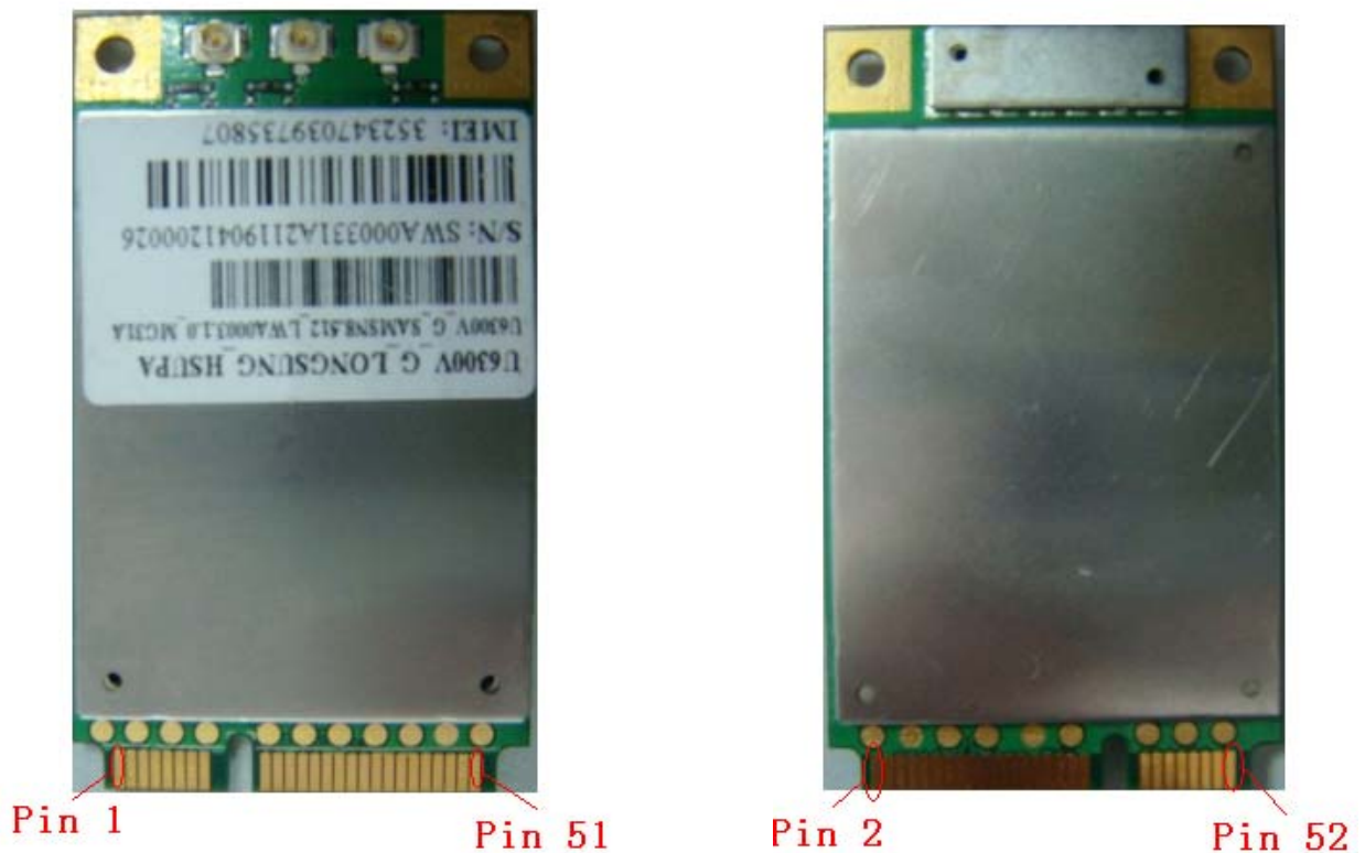
Figure 2-5 The Mini PCIe Interface pin sequence of U6300
