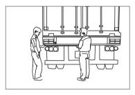
Installation height for sensor can be adjusted,2.5-4.0ft vertically high to the ground
