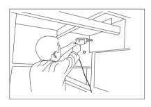
1. Choose suitable control box position, then punching in the corresponding position.
