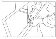
Connect the power line of control box and power source of reversing light
