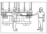
3 Measure the distance 0.5-0.65f on its side for position A&D, between sensor A&D get the result "L", mark sensor B&C for every 1/3 "L"interval.
