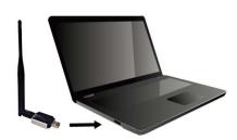
After the computer has fully rebooted, locate a USB port and insert the USB Adapter. Windows should automatically begin to install the driver for using the USB Adapter.
