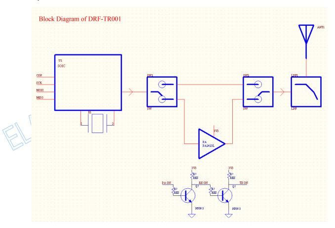
The SPI data then is fed to SOIC for encoding, FSK-modulation, frequency conversion, and amplification.
