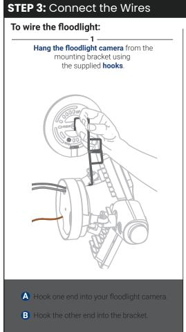
The copper wire from the camera is ground wire.
