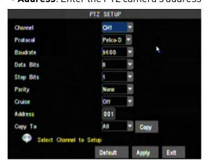
Use the Copy To drop-down menu to copy the PTZ settings to multiple channels.
