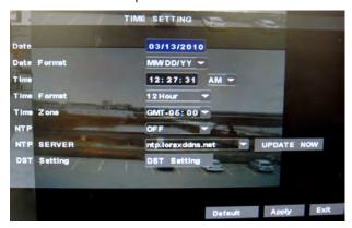
If the system will not have access to the internet, you must manually configure DST by clicking the **DST Setting** button. For details, see "Adjusting the system time and DST (Daylight Saving Time)
