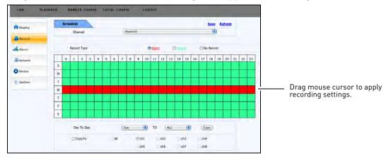
In this example, Alarm recording was applied to all 24 hours of Wednesday (the grid highlights in red). The remaining days are in "Normal" recording mode (the grid highlights with a light green).
