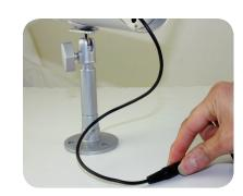
Connect power adapter to local 120V AC power outlet
