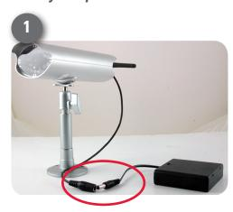
1. Connect camera to the Battery Adaptor.
