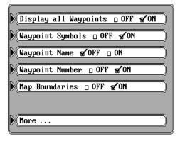
"More..." label. The screen shown at the bottom of the previous page appears. Press the key next to the desired option, then press the CLR key to exit this screen.
