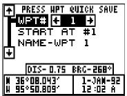
You can select any waypoint as the simulator's starting point. Select the starting point by pressing the right arrow key on the "WPT#" label until the desired starting waypoint number appears. Now highlight the "Start At" label and press the right arrow key. The GlobalNav 310 returns to the Simulator Setup menu.
