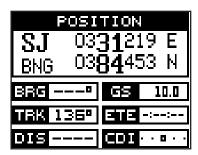
The GlobalNav 310 can use the military grid reference system (MGRS). It uses two grid lettering schemes, which are referred to as standard and alternate MGRS on the GlobalNav 310. Your position and datum in use determines which one to use. In general, if the datum you're using is valid for your present position, then use the standard MGRS, otherwise use the alternate MGRS.
