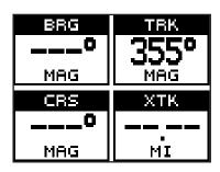
ror (XTK) are all shown on this screen. You must recall a waypoint to use the bearing, course, and cross track error windows. As you wait for it to find your position, you'll see numbers flashing on the display. Anytime you see flashing numbers, it means the GlobalNav 310 does not have a position! Do not rely on any data that is flashing! When the numbers stop flashing, the unit has locked on to the satellites and the position is good.
