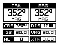
This screen is composed of eight digital display boxes, showing your track (TRK), and ground speed (GS). The other boxes show navigation data when a waypoint is recalled, including bearing to the waypoint (BRG), course (CRS), Altitude (ALT), distance to waypoint (DIS), velocity made good (VMG), and cross track error (XTK).
