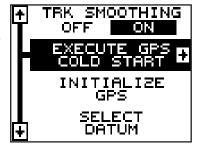
To view these menu items, press the MENU key, then highlight the "GPS Setup" menu. Press the right arrow key. The screen shown above appears.
