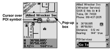
At left, an iFINDER GPS screen showing a POI pop-up name box. At right, you can call up a page of information on the POI, and the GPS unit can lead you to the POI's location.
