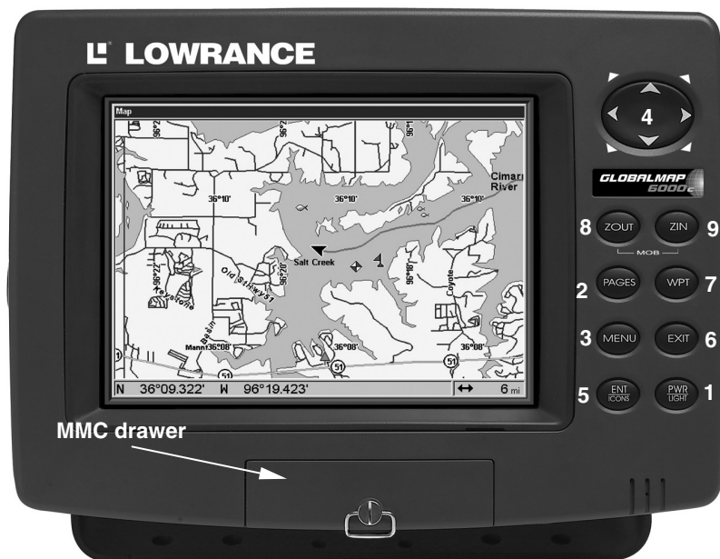
GlobalMap 6000C GPS unit, front view, showing screen, keyboard and MMC drawer.
