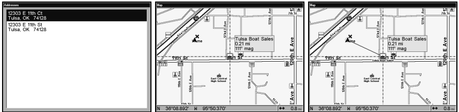
Address search result list, left. At center, Map Page showing location of the address on the map, highlighted by cursor. At right, after the address is located, you can navigate to it.
