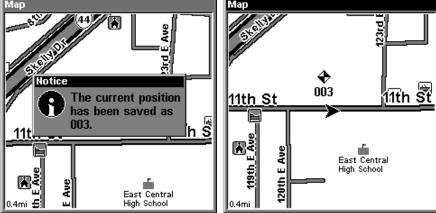
Sequence for setting a waypoint. Step 1: while traveling, *quickly* press WPT *twice* to call up Find Waypoint screen (seen in Step 2) and set a point. Step 3: a message says the waypoint has been saved. Step 4: vehicle continues on its way; number waypoint symbol is visible on map.
