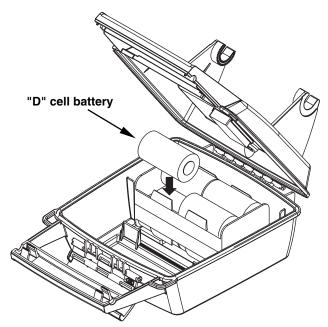
Install batteries in power pack battery adapter.
