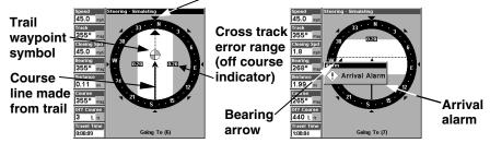
Navigate trail, navigation page (compass rose) views: at left, driver is northbound heading straight toward trail point 6; bearing arrow shows the trail point is due north (straight ahead.) At right, driver has reached trail point 6 and must turn west to follow the trail. Arrival alarm goes off and bearing arrow swings around to say turn left (west), toward the next waypoint, trail point 7. LMS-320 now shows navigation information to point 7, which is 1.99 miles away.
