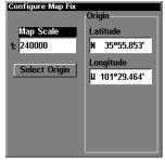
Configure a map fix so LMS-320 can find your position on a printed chart or topographical map.
