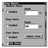
Sonar Alarms menu with Fish Alarm selected. The check box to the left is blank, indicating the alarm is turned off.
