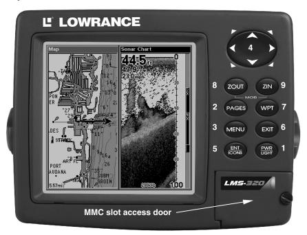
LMS-320 series sonar/GPS unit, front view, showing map with sonar split screen, keyboard and access door for the MMC slot.
