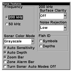
Sonar Features menu with a frequency of 200 kHz selected. To change the frequency setting to 50 kHz:
