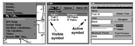
Sequence for saving a trail and beginning a new one. At left, My Trails command. Center, the Trails Menu. The arrow to the right of Trail 14 indicates the trail is "active," and the check to the left indicates the trail is visible on the map display. The right figure shows the Edit Trail menu, with the Active command selected.
