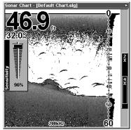
At left, Sonar Menu with Sensitivity command selected. At right, the Sensitivity Control Bar.
