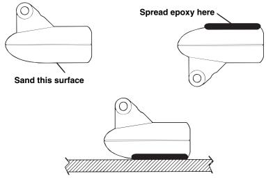
Epoxy transducer to hull.
