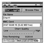
At left, the Sonar Page menu with the Log Sonar Chart Data command selected. At right, Sonar Chart Logging menu, with the Start Logging command selected. The menu says the MMC has 5.42 MB of free space, which will record the scrolling chart for 28 minutes and 44 seconds.
