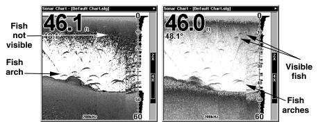
Sonar chart in regular grayscale mode, left, and in FishReveal mode, right. Notice how shallow fish formerly hidden in the surface clutter become visible in FishReveal mode.
