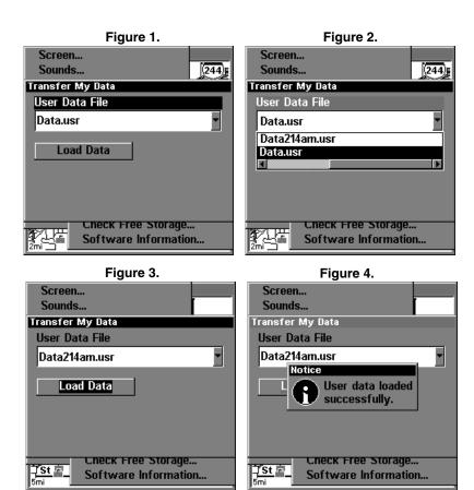
These figures show the menu sequence for loading a GPS Data File from an MMC into LMS-320's memory.
