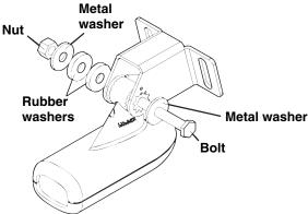
Assemble transducer and bracket.
