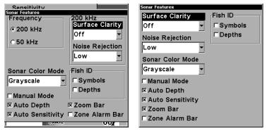
Sonar Features menu with Surface Clarity selected (at left, dual-frequency menu; at right, single-frequency menu).
