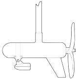
Transducer mounted on trolling motor, side view.
