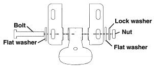
Assemble transducer and bracket.
