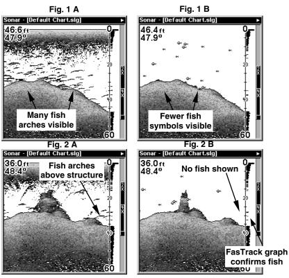
At left, figures 1A and 2A show Sonar Page in normal chart mode. At right, figures 1B and 2B show the same underwater scene with Fish I.D. turned on. Note how arches are replaced with symbols.
