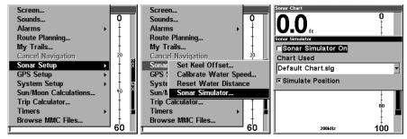
At left, Main Menu with Sonar Setup command selected. Center, submenu with Sonar Simulator command selected. At right, Sonar Simulator menu, with simulator turned off (check box is unchecked).
