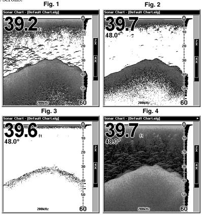
These figures show results of different sensitivity levels on the same location. Fig. 1: Sensitivity at 88 percent, determined by Auto Sensitivity. Typical of full auto mode. Fig. 2: Sensitivity set at 75 percent. Fig. 3: Sensitivity set at 50 percent. Fig. 4: Sensitivity set at 100 percent.
