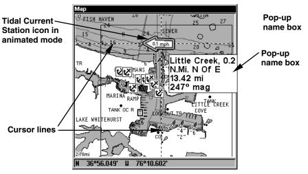
Navionics chart showing Tidal Current Station icon selected by cursor. In this example, the tidal current is in flood but it's about to enter the slack water stage. The current is flowing to the west at 0.1 mph.
