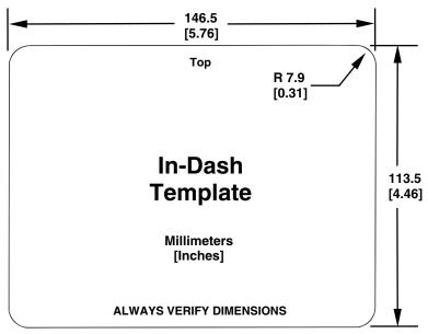
In-dash mounting template for LMS-320 sonar/GPS unit, showing dimensions. NOTE: The figure above is *not* printed to scale. A scaled template (FM-5 In-Dash Adapter Kit instructions) is available for free download from our web site, www.lowrance.com.
