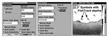
Sonar Features menu with Fish I.D. Depths selected (at left, dual-frequency menu; center, single-frequency menu). When the check box to the left is checked, the feature is on. At right, Sonar Page showing Fish I.D. symbols and FishTrack depths turned on.
