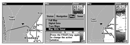
Map With Sonar split screen option. At far right, the full Map Page is shown. The Pages Menu with the Map option list is shown in the center. At right, the Map With Sonar split screen is shown.
