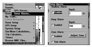
At left, Main Menu and Sonar Alarms command. At right, the Sonar Alarms menu.
