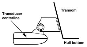
Align transducer centerline with hull bottom.
