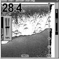
At left, Sonar Menu with Ping Speed command selected. Ping Speed Control Bar, right, at default setting.
