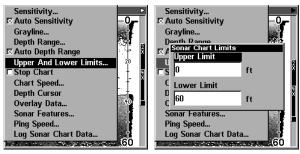
At left, Sonar Page Menu with Upper and Lower Limits command selected. At right, Sonar Chart Limits menu, with Upper Limit selected.
