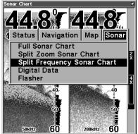
Split Frequency Sonar Chart page, with 50 kHz view at left and 200 kHz view at right.
