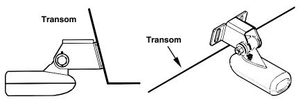
Position transducer mount on transom and mark mounting holes. Side view shown at left and seen from above at right.
