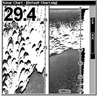
Split Zoom Sonar Chart. Image at left shows the left window zoomed to 2X. The right image shows the left window zoomed to 4X. The depth overlay data is set to the default large text size; the water temperature is set to the small text size.
