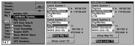
Menus for changing coordinate system used to display positions.
