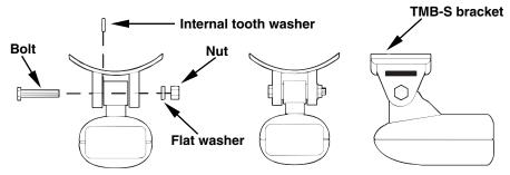
Attach motor mounting bracket to transducer.
