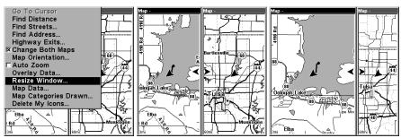
At left, Map Menu with Resize Window command selected. Center, Resize Window command is active. At right, pressing the → key moves the centerline to the right and enlarges the left window.
