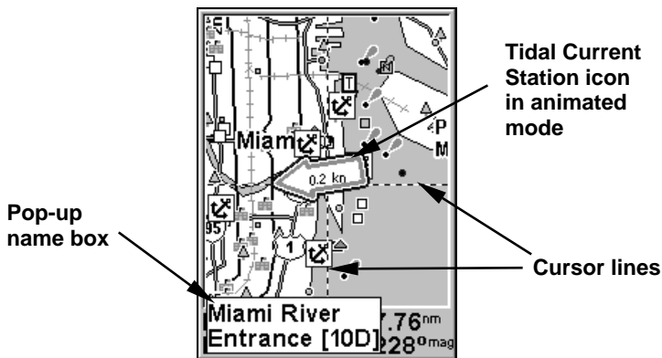
Navionics chart showing Tidal Current Station icon selected by cursor. In this example, the current is flowing to the west at 0.2 kn.
