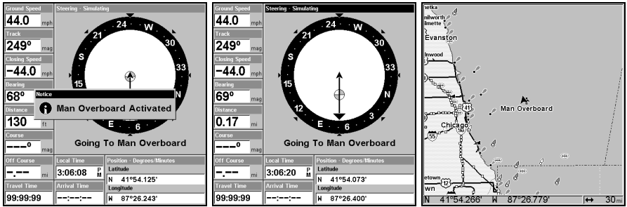
Navigating to Man Overboard: Man Overboard Activated message, left, Navigation Page, center, Map Page, right. The victim is to the starboard of the vessel; the GPS shows which direction to steer to for the rescue.
