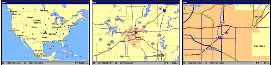
Map Page opening screen (left). Zoomed to 100 miles (center) and zoomed to 15 miles (right). Over Zoomed means you have reached the detail limits in an area covered only by the basic background map. Zooming in any closer will reveal no more map details because a high-detail custom map has not been loaded on the MMC.
