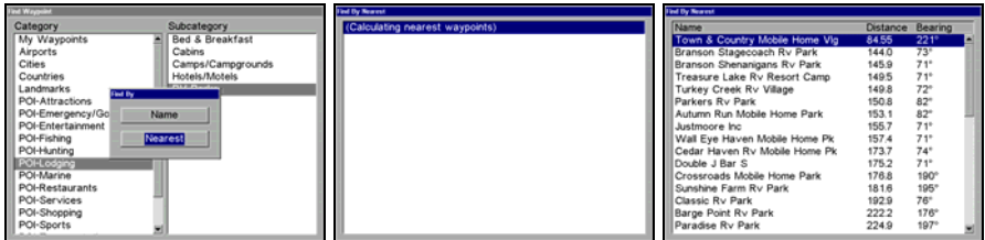
Find by Nearest option (left) with Calculating screen (center) and POI list (right).
