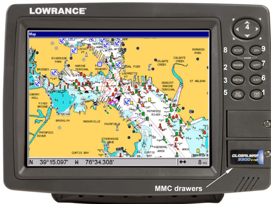
GlobalMap 9300CHD GPS unit, front view, showing screen, keyboard and MMC drawers.
