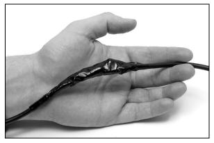
After taping the wire ends individually, wrap the entire connection with electrical tape as shown. This will help protect from moisture and prevent the wires from breaking contact.
