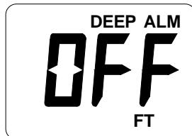
The alarms are now set. If you move into water shallower than the shallow alarm's setting or deeper than the deep alarm's setting, the appropriate alarm will sound.
