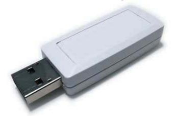
The CORE USB dongle from LumenRadio provides a commissioning interface for a CORE mesh network that can be quickly and easily connected to a host computer. For Linux and MAC users no extra drivers are needed.
