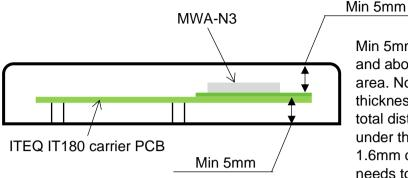
Min 5mm to solid objects under and above MWA-N3 antenna area. Note that carrier board thickness can be included in the total distance to solid objects under the antenna. I.e. for a 1.6mm carrier board standoffs needs to be min 3.4mm
