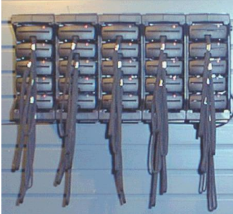
25 keypad wall mounted charging rack
