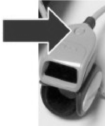
Figure 1-34 Scan Status LED
