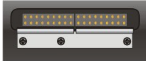
Figure 1-5 Scanner / Audio / Battery Ports – Connector 1 and 2
