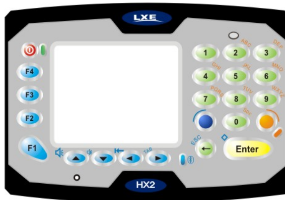
Figure 1-26 The 23 Key Keypad (Default)
