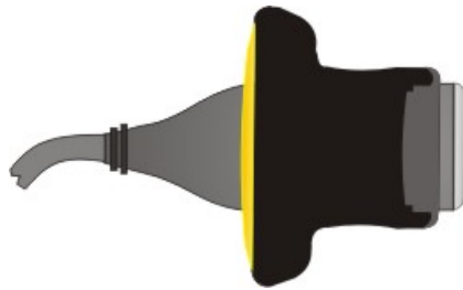
Figure 1-42 Step 2 : Rotate Trigger Module again until it pops up. Remove the trigger module.
