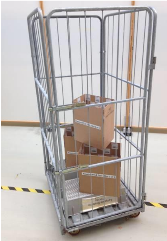
Figure 13. A roll cage with test tag cartons placed on a plastic box.
