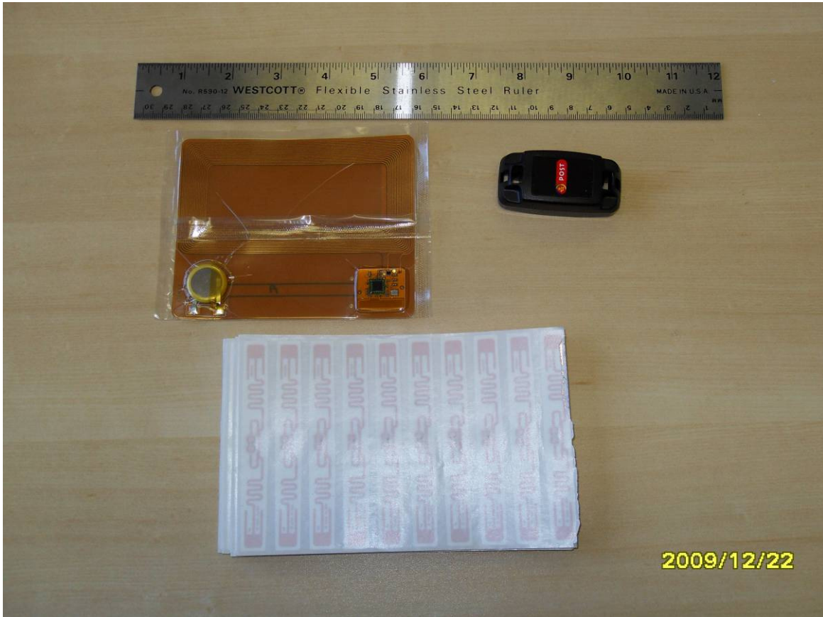
Figure 10 – Active and Passive RFID tags
