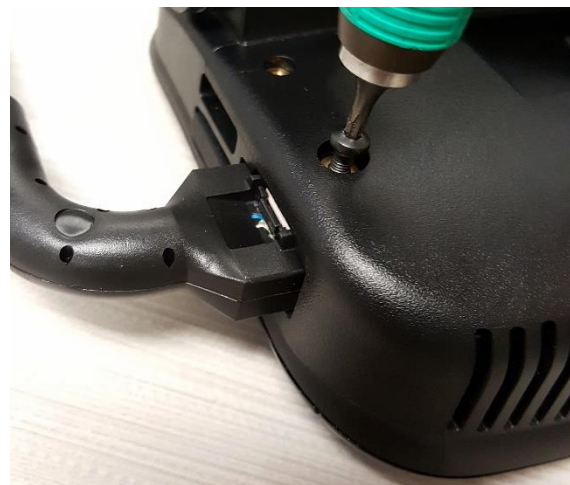
ER-SF1 Locking Tab with T8 Security Screw
