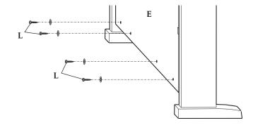
Turn the adjustable Pedal Board support, until it is in firm contact with the floor.
