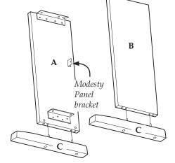
Place the cylindrical nuts (G) in the holes near the lower bracket in each leg (A and B), with the Phillips slots (+) facing up for each nut.
