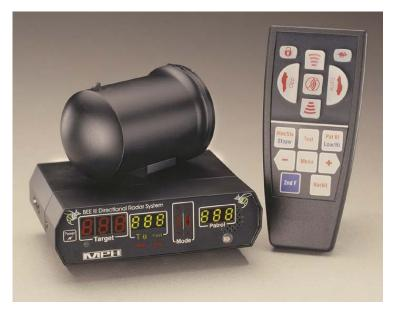
The BEE III employs state-of-the-art digital signal processing (DSP) technology, which allows the unit to have both high performance and high reliability in a small package. The digital signal processor is a specialized microprocessor chip, which can perform the required calculations for detecting patrol and target speeds very efficiently.
