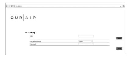
4. Enter Wi-Fi Encryption information and click save to save your settings. The device will restart to complete the Wi-Fi configuration. If the front LED is on, the Wi-Fi is connected successfully.
