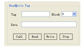
Specify: before run READ, WRITE, CALL function, must input this tag ID number in "Select TAG" bar, then start operating the tag.
