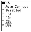
Setting the time until automatic reconnection, when the connection is lost.
