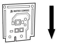
3. Lower the module in this position into the CPM slot as shown in Fiure.
