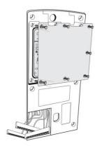
2. Hold the Card Personality Module with the smooth surface towards you, and the narrower end facing down as shown in Figure.
